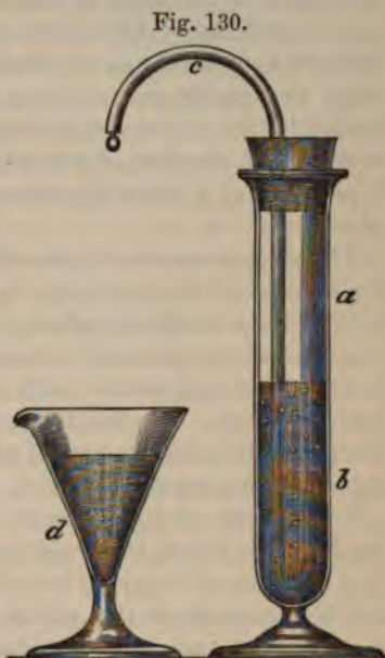
FERMENT-APPARATUS, containing saccharine urine in fermentation.— a . Upper part of the test-tube containing carbonic acid. b . Lower part of the test-tube containing the fermenting liquid. c . Bent glass tube, to allow the escape of liquid. d . Liquid which has been forced out from the test-tube by the accumulation of gas.
